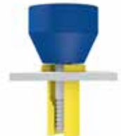
2. Place the loaded tool into the pre-drilled hole in the wishbone arm.
