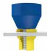
3. Operate the tool to place the rivet nut into place
