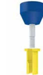
1. Screw nut onto a blind rivet nut placement tool.
